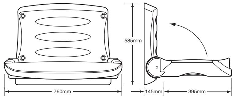
Suggested mounting height from the floor to the base of the unit is 730mm
